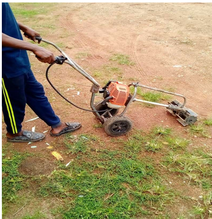
Figure 2. Mechanical weeder with protected exhaust pipe
