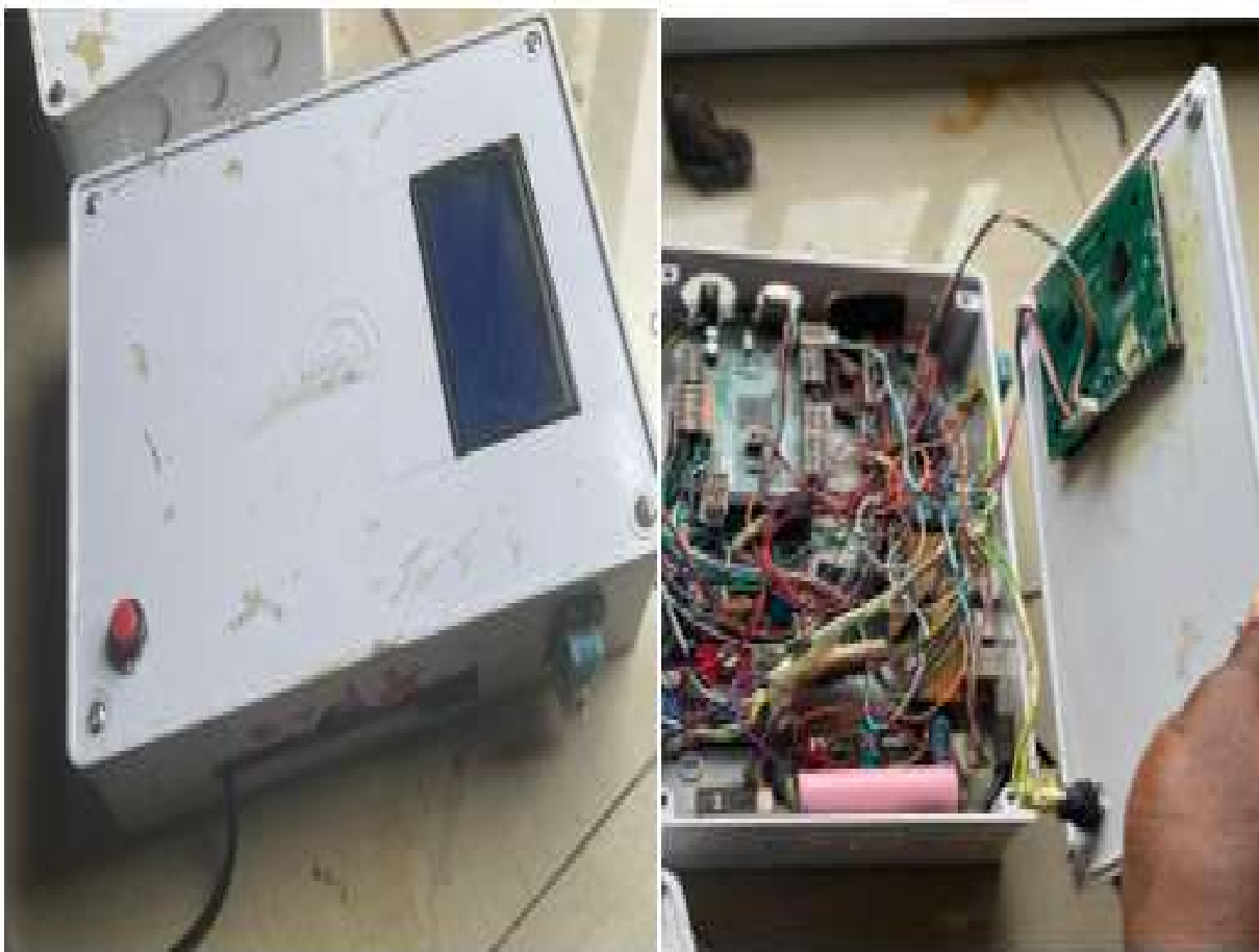
Figure 4: Plastic housing for microcontroller, display and other units
